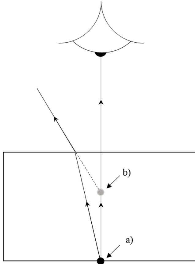
*Fig. 9. Construction of virtual image formed by ordinary rays. a) is location of point-like object; b) is location of its image.*
