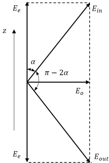
Fig. 11. Rotation of linear polarization by means of half-wave plate.
