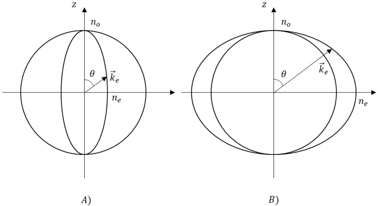
Fig. 6. Refractive index ellipsoid cross section
