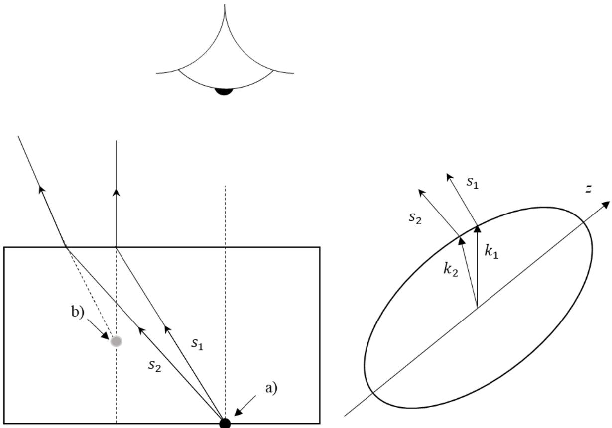
*Fig. 10. Constructing image formed by extraordinary rays. a) is location of point-like object; b) is location of its image.*
