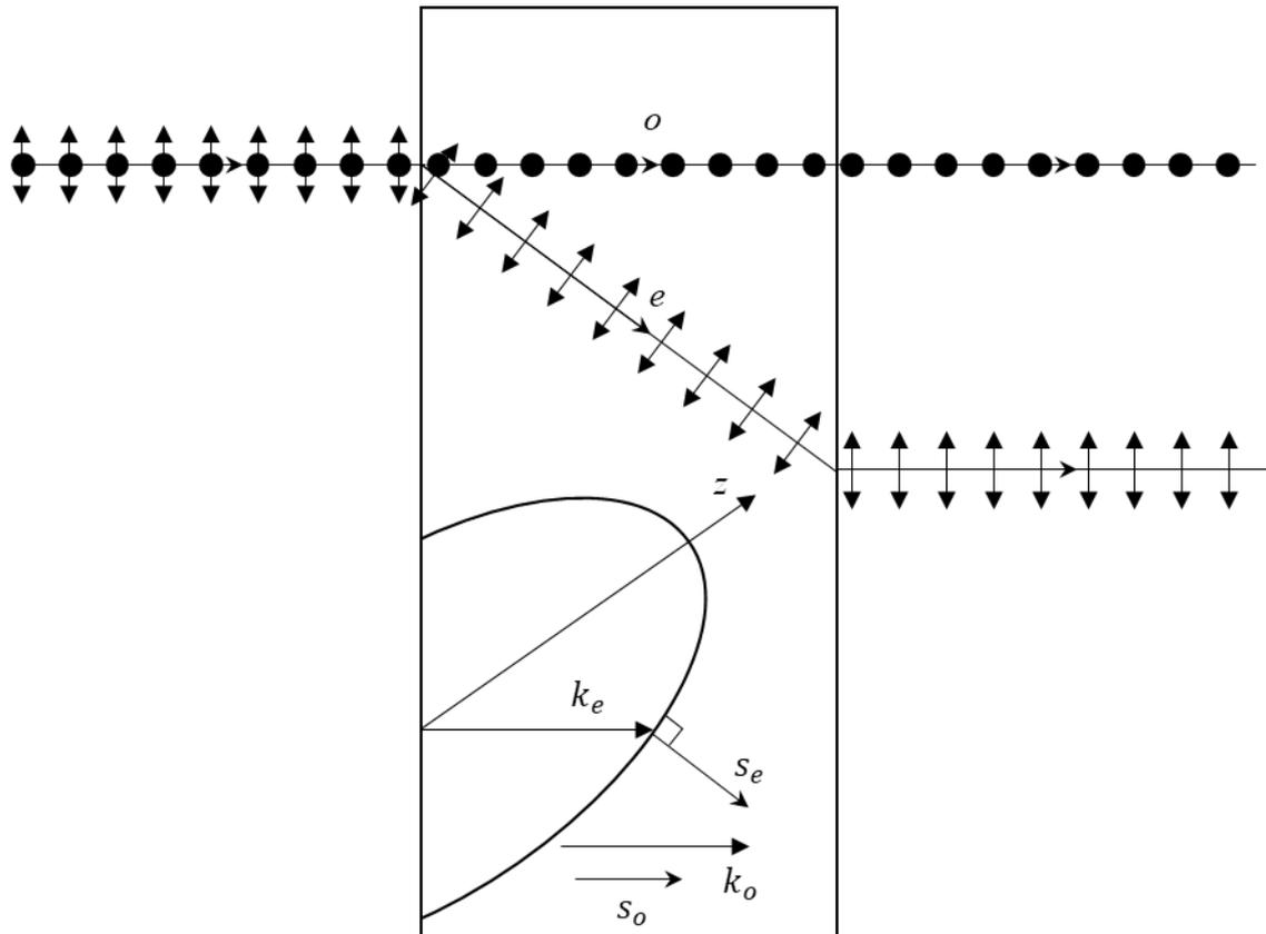
Fig. 8. Walk-off of rays in uniaxial crystal at normal incidence.
