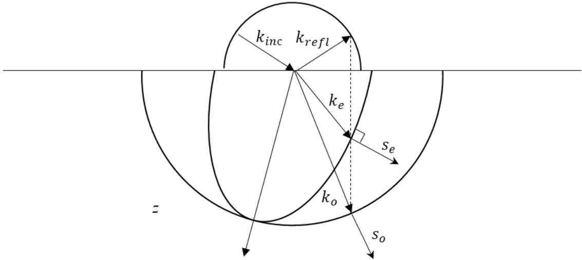
Fig. 7. Finding out directions of propagation of refracted rays in uniaxial crystal.
