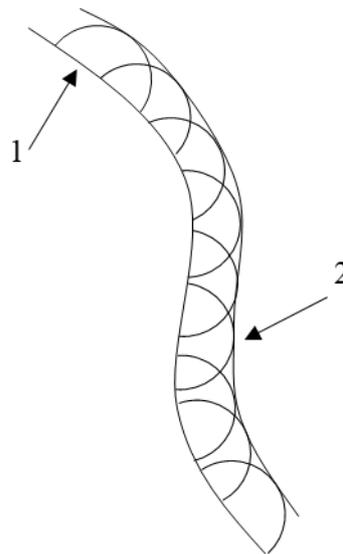
*Fig. 3. Huygens method of constructing wavefront by using secondary sources.*
