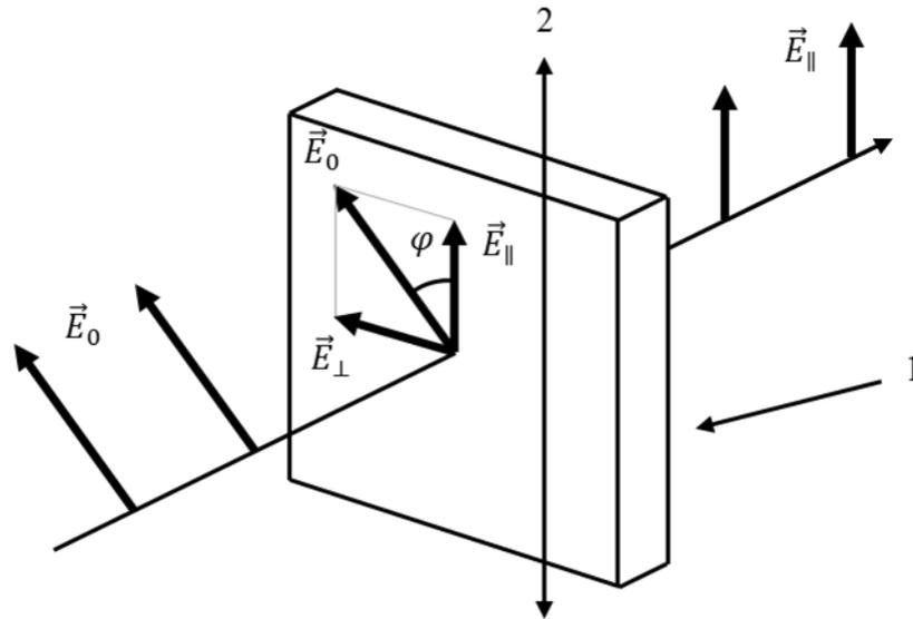
Fig. 2. Passing of light through linear polarizer.
