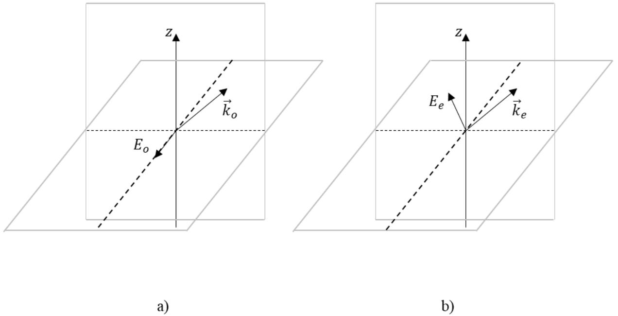
Fig. 5. a) Direction of electric field vector of ordinary wave;
