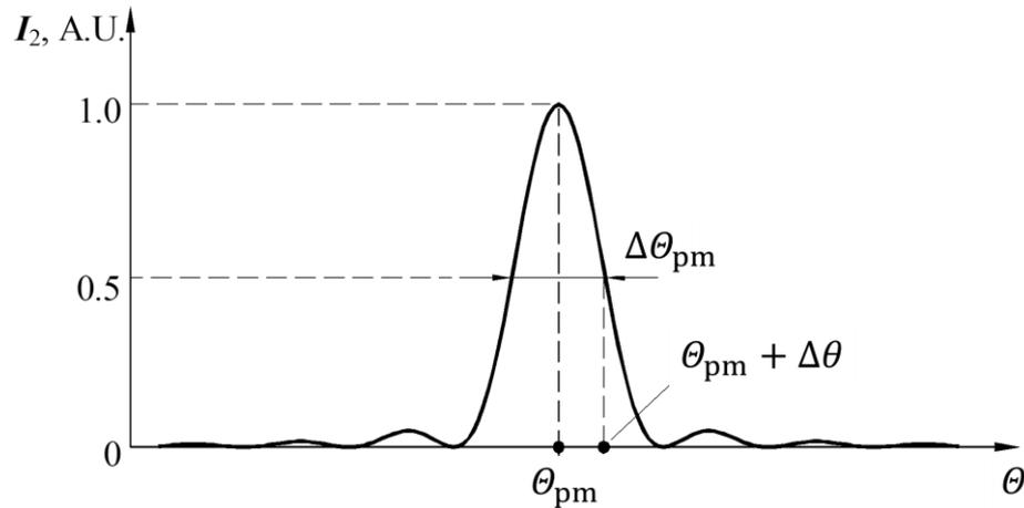
Fig. 8. Intensity of the second harmonic versus angle.
