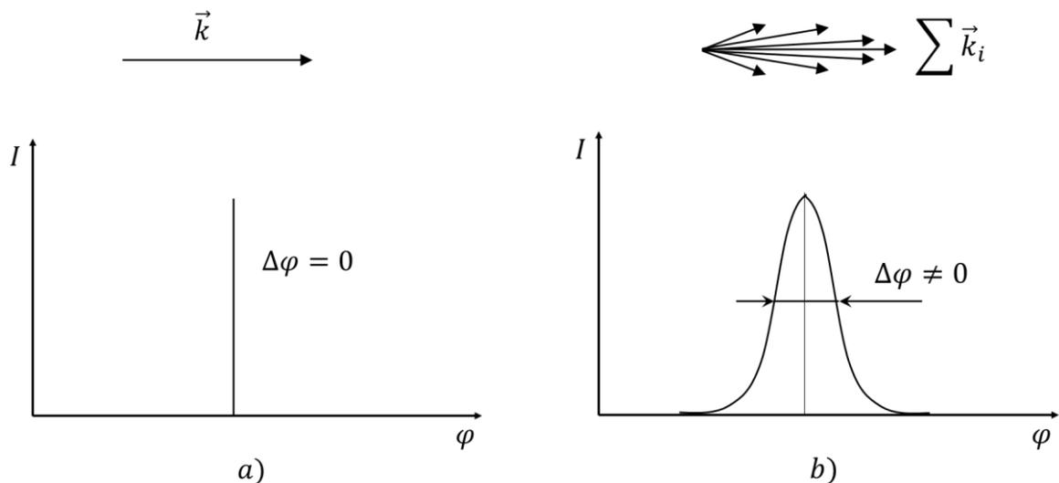
Fig. 9. Angular divergence of plane wave (a) and real beam (b).
