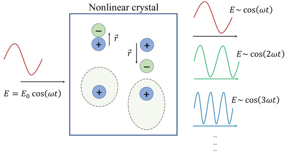
Fig. 4. Generation of optical harmonics in nonlinear medium.
