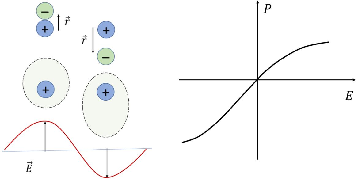
Fig. 3. Emergence of nonlinear polarization in asymmetric medium.
