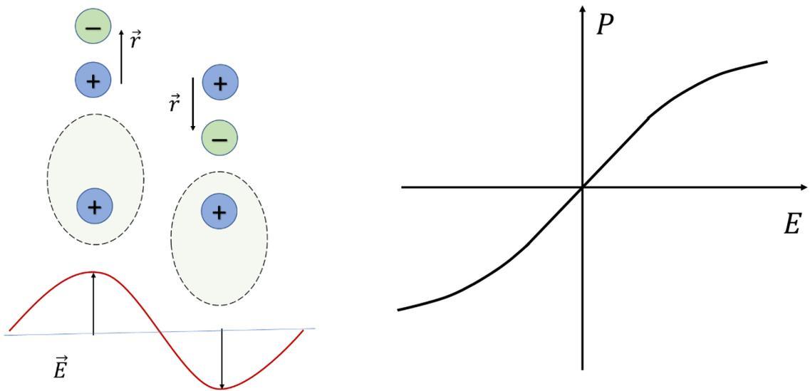
Fig. 2. Emergence of nonlinear polarization in isotropic medium.
