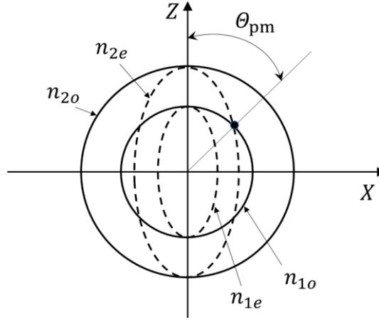
Fig. 7. Cross sections of refractive index surfaces for positive a) and negative b) crystals.
