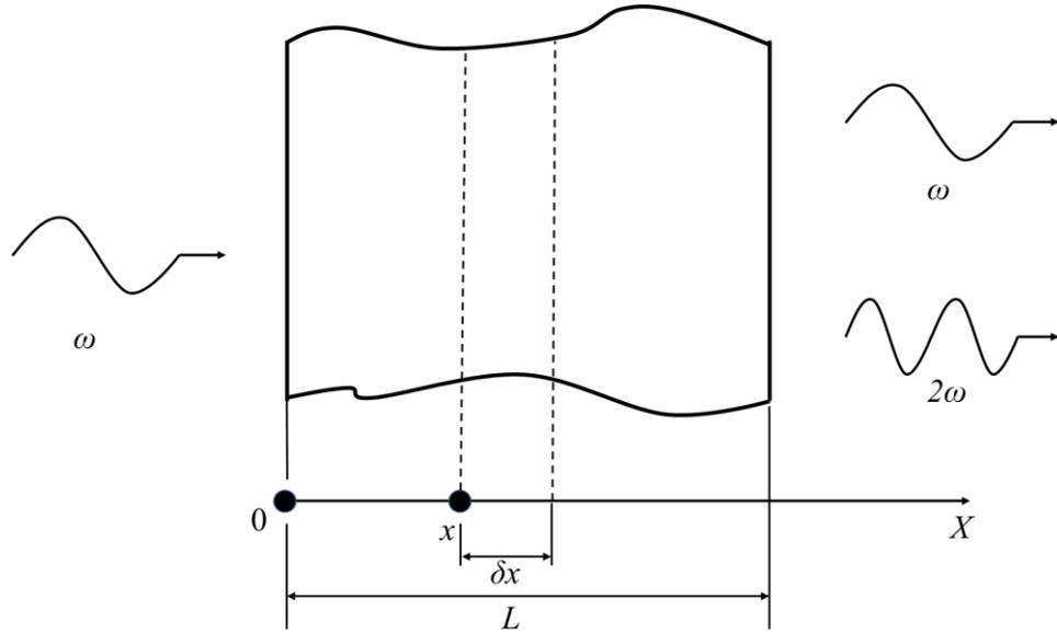
Fig. 5. Generation of the second harmonic in nonlinear crystal.
