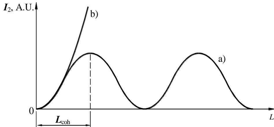
Fig. 6. Intensity of the second harmonic  $I_2$  versus length  $L$  of nonlinear crystal:
