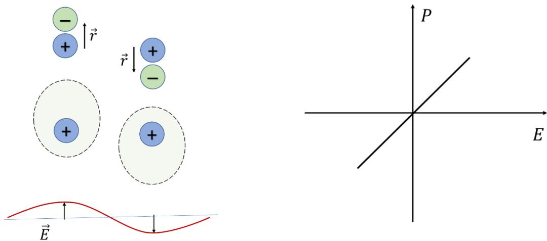
Fig. 1. Generation of linear polarization in matter.
