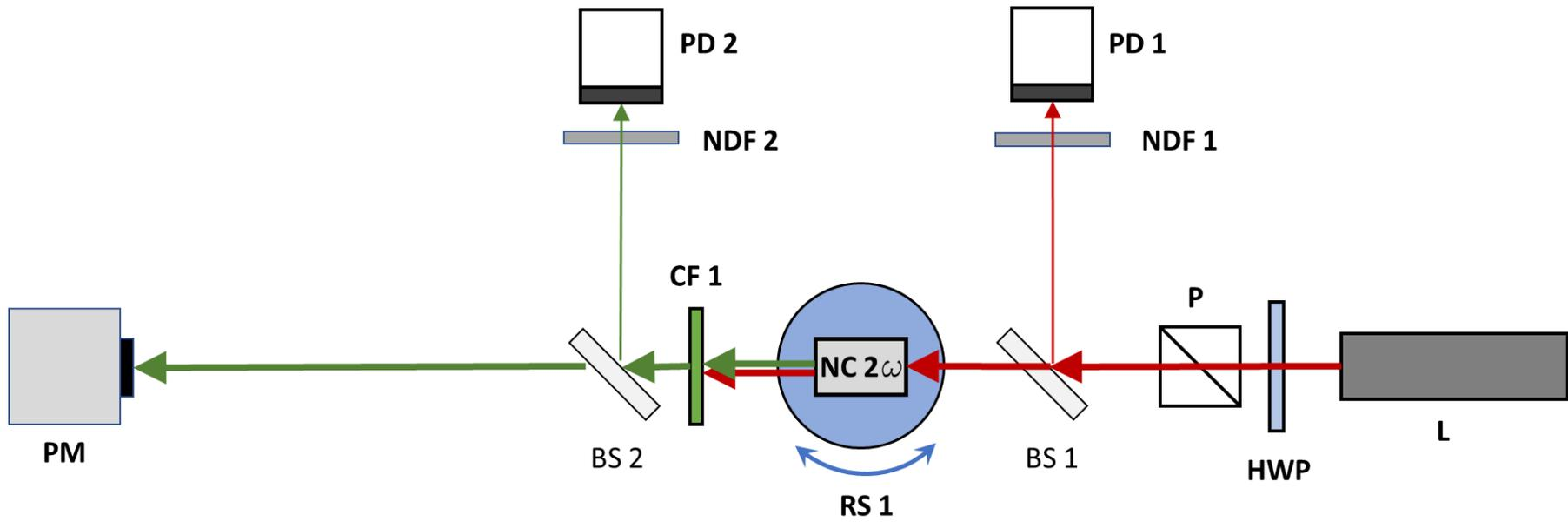
*Fig. 1. Experimental setup for study of generation of the second harmonic.*
