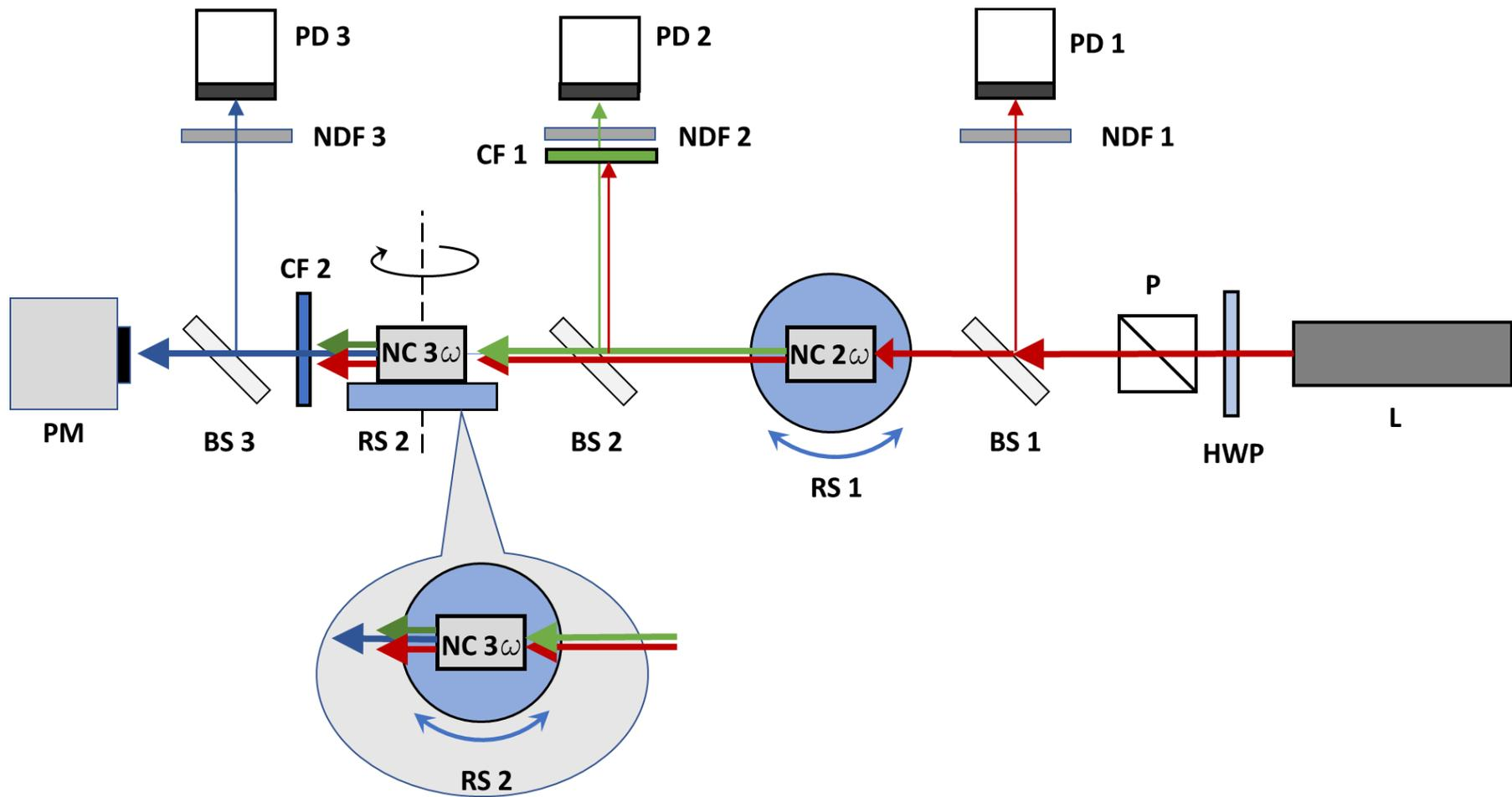
Fig. 2. Experimental setup for study of cascade generation of the third harmonic.
